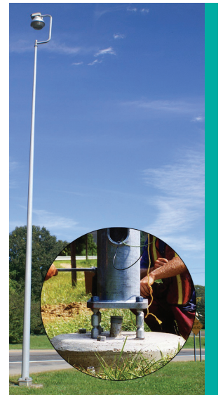
Figure 25. An Omnidirectional Breakaway Support System for Light Poles (Image: Transpo 2014)
